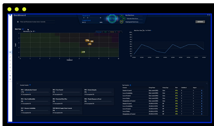
Top attack scenarios for different business processes, detailing the likelihood, impact and risk factor for each
